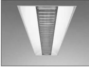
**Applications:** The SYNTO family of fixtures combines indirect illumination with a direct component controlled with a T5 louvre to minimize brightness. The Zumtobel Staff exclusive light chamber provides soft and diffuse general illumination; the louvre has been specifically developed to minimize glare when using T5 lamps. This solution is best for open offices, retail spaces and institutions.
